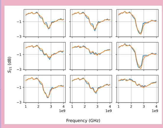
Actual responses (blue traces) and predicted responses (orange traces) for the scattering coefficient data  $(S_{21})$  originating from various unseen magnetic microwire tag configurations.
